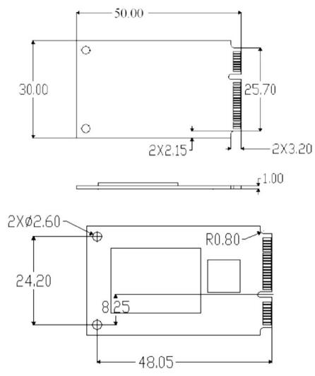
The module extends 2.3mm above the mini PCI express board. Hence total module thickness is 3.3mm.
